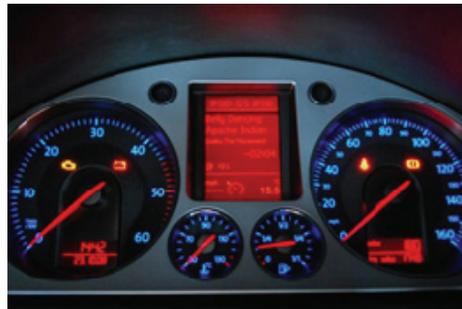
The menu of the Gateway Pro is displayed on the central display (cluster) on the dashboard (between the two main instruments). Due to the capabilities of your car, the Gateway Pro menu is **not visible** on the **radio screen**.
