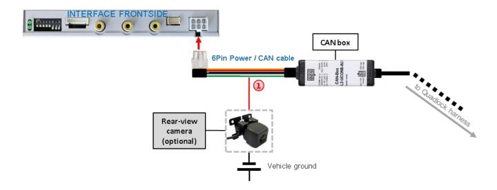
1 The 12 V power supply for the rear-view camera (max 3A) has to be taken from the green wire of the 20pin cable to avoid an unnecessary permanent power supply to the camera electronic.
