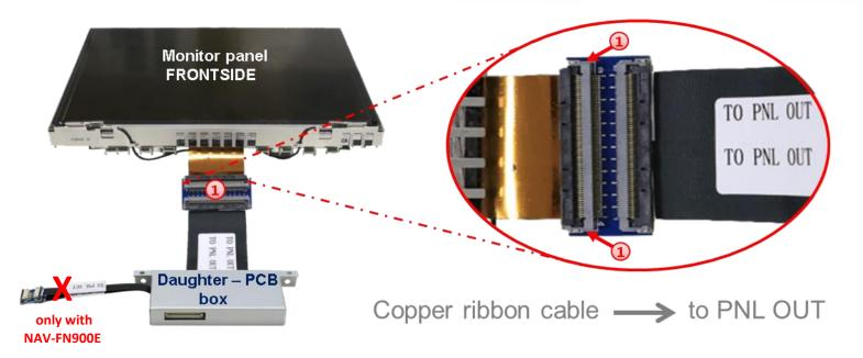
1 Turn around the monitor panel and connect the previously become free copper coulored 60pin ribbon cable to the pre-assembled 60pin ribbon cable merger "TO PNL OUT" of the daughter PCB box and clip it in (heed the following warning notes!).
