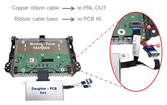
1 Click out the copper coloured 8pin ribbon cable from the monitor mainbord's ribbon cable base, connect it to the daughter PCB's 8pin ribbon cable merger PNL OUT and lock it's closure.
