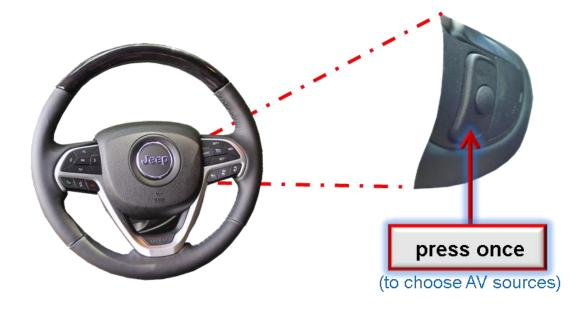
A press of the volume button on the right rear side of the steering wheel switches the input from factory mode to the inserted video sources. If -by dip switch setting- all inputs are enabled, the order will be the following:
