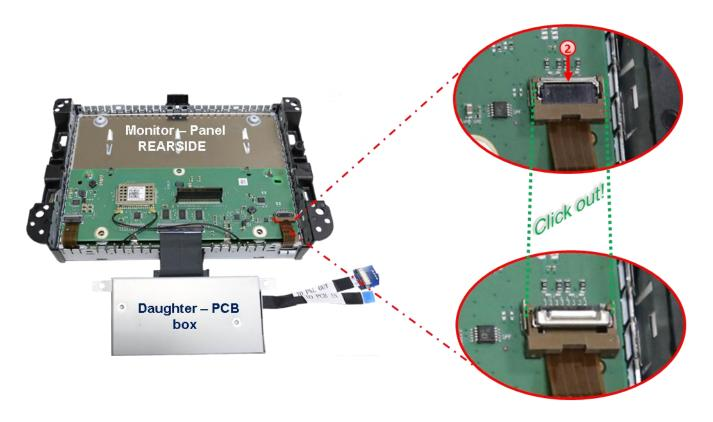
Carefully unlock and pull back the 8pin touch ribbon cable base closure on the right side of the monitor motherboard like shown in the picture.
