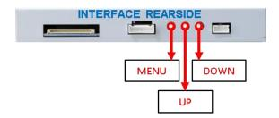
The picture settings are adjusted by the 3 buttons on the video-interface. Press the MENU button to open the OSD settings menu. To switch to the next menu item, pressing UP and DOWN will change the selected value. The buttons are embedded in the housing to avoid accidental changes during or after installation. The picture settings have to be done separately for RGB, AV1 and AV2 while the corresponding input is selected and visible on the monitor.
