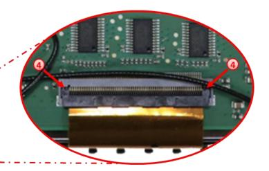
4 Carefully clip out the kopper coulored 60pin ribbon cable at the monitor panel's ribbon cable base and lead it out.
