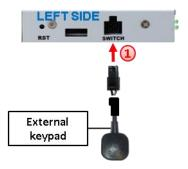
1 Connect the external keypad's female 4pin connector to the video-interface's male 4pin connector.
