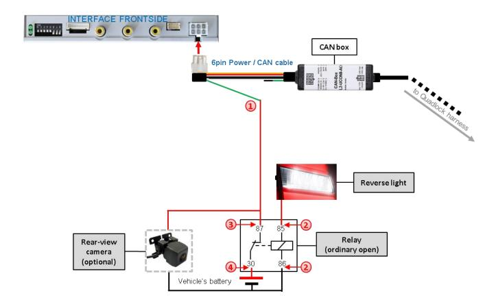
① Cut through the 6pin Power / CAN cable's green cable and connect the one side which is near to the 6pin Power /CAN connector to the output connector (87) of the relay.
