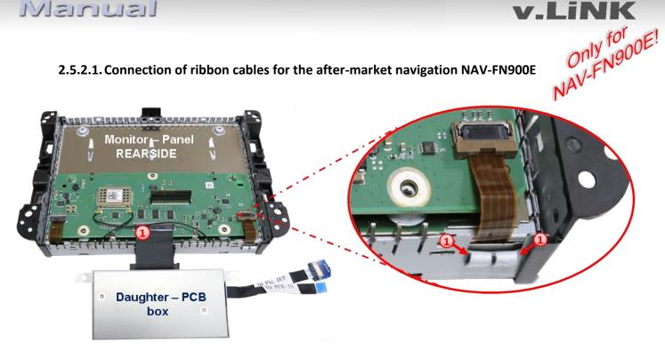
(1) For leading out the 8pin touch ribbon cables out of the monitor housing, both metal sheet tabs underneath have to be bent down to avoid a cable injury with later reassembly of the housing parts. Further, for saving the ribbon cables, the down bent sheet tabs should be covered with a piece of smooth tape.
