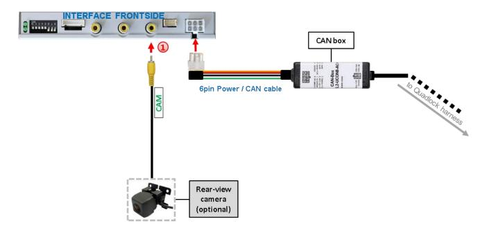
Connect the video-RCA of the after-market rear-view camera to the female RCA port "CAM" of the video-interface.
