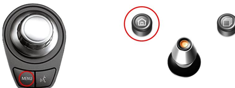
In **BMW** in the vehicle's **Entertainment** menu activate **AUX** and in **Mini** in the vehicle's **CD/Multimedia** menu, activate **AUX front** by iDrive and after it **long press MENU** button (1- and 2-button iDrive + Mini) to choose the interface as current AV-source.
