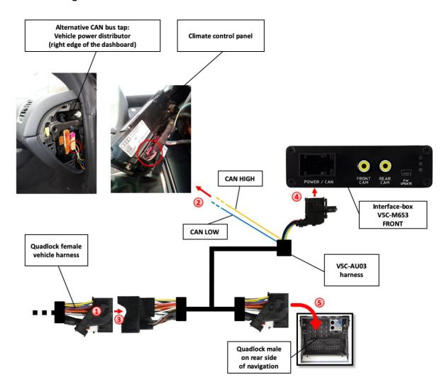
Remove the female Quadlock connector of the vehicle harness from the rear of the navigation computer.
