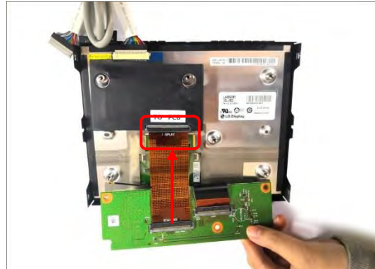
8、 OEM 68P inserted to the daughter PCB's socket.
