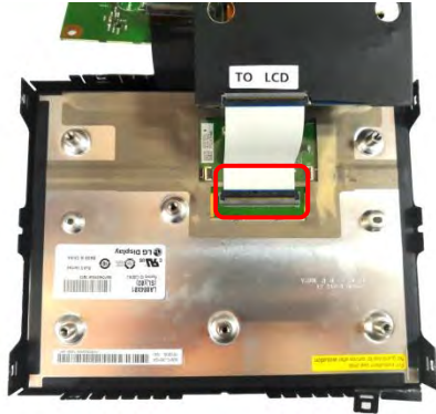
7、 the daughter PCB's 68Pin ribbon insert back the the OEM socket.
