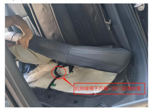
Install suction lock and fix it, connect original connectors to our special connectors.
