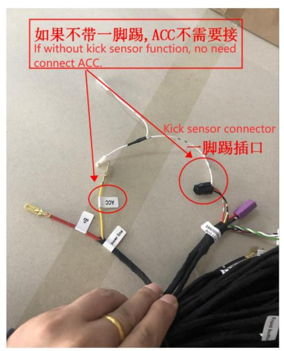
Above positions are the wiring diagrams of some models. After installed pole and lock, please open and close door manually, make sure that not have any scratches. Then make power and signal testing, if working correctly, then wiring all sets.
