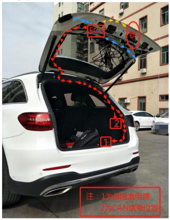
After installation, power on and close the tail door manually, test the product to check whether the pole is pressed, the ball head gasket can be fine-tuned, you can use our development center HOOK & LOOP and tie to fix control box and wirring, install each parts as where they are, the installation is complete!
